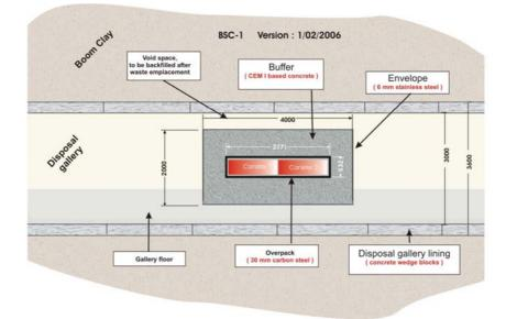
Figure 1. The disposal gallery design for vitrified high-level waste
